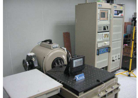
Operating Vibration Test - X axis
