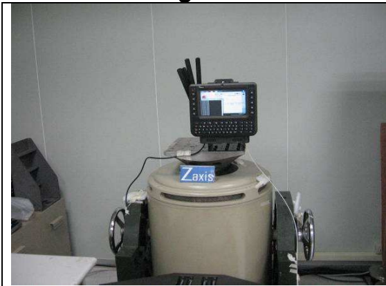
Operating Vibration Test - Z axis
