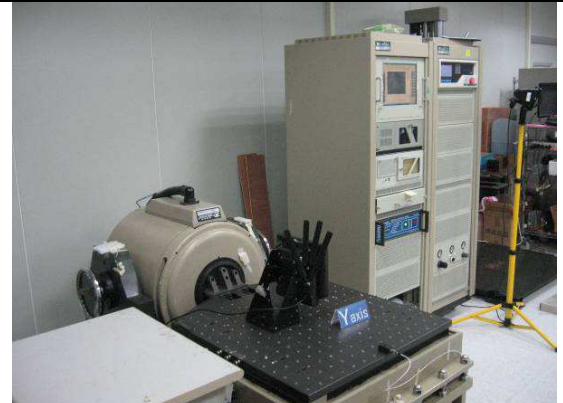
Operating Vibration Test - Y axis
